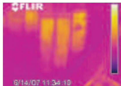
Missing or settled insulation
