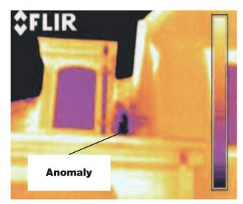
Without *Masterpiece* HomeScan, the owner of this home would not notice the beginning of a leak in what appears to be a fully functioning roof (above left). The dark colors next to the window in the HomeScan image (above right) indicate the presence of water collecting under the roof. Detecting what the naked eye can't, HomeScan uncovers this problem long before it becomes a major issue.
